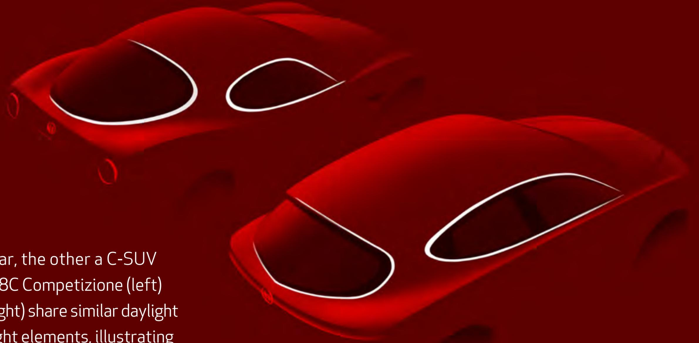
One is an exotic sports car, the other a C-SUV concept. The Alfa Romeo 8C Competizione (left) and the Tonale concept (right) share similar daylight opening (DLO) and backlight elements, illustrating the connection of Alfa Romeo design themes across vehicle types and segments.
