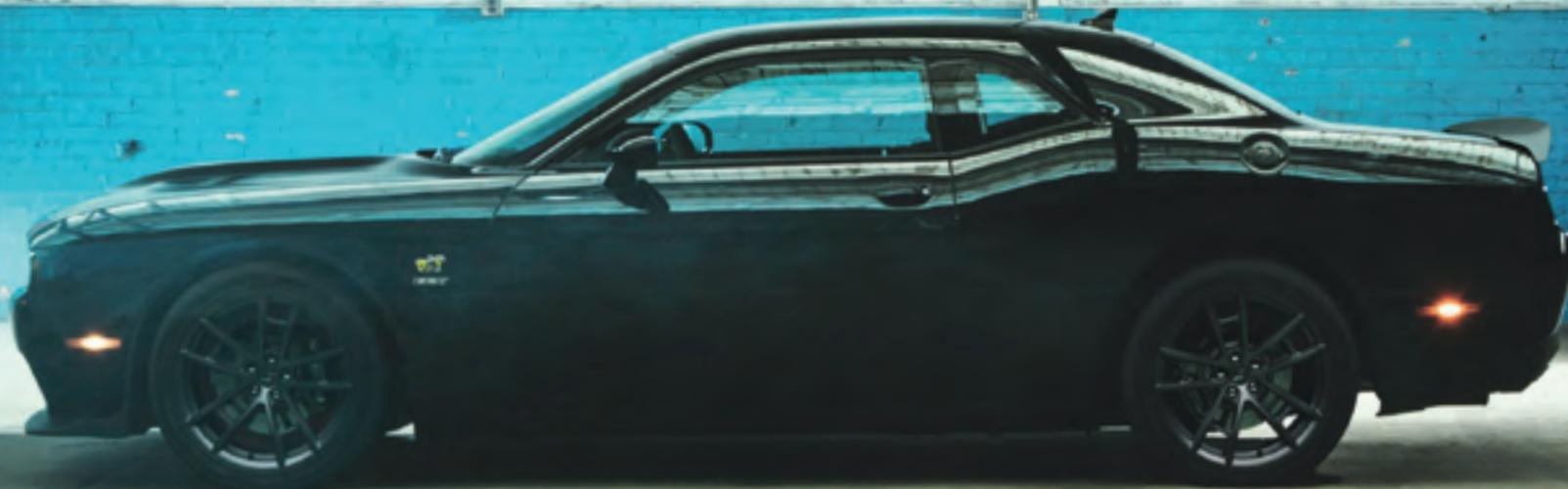
Subtle isn't what this car is about. It was conceived to live its best life on the drag strip. Its purpose is maximum acceleration. It's outfitted with everything needed to floor it on the last yellow: TransBrake, drag suspension, Adaptive Damping Suspension, 275/40R20 102Y Drag Radial tires and 20 by 9.5-inch Low-Gloss Black drag wheels with knurled bead seats. This is the 1320, and it's only available on R/T Scat Pack. The unique fender badge lets everyone know you aren't messing around;
