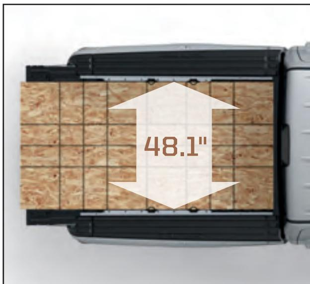
**STANDARD SHEETS FIT.** Opting for the available RamBox® System doesn't mean sacrificing precious bed space. You'll still have plenty of room to carry wide cargo, like standard 4x8-foot sheets of building materials.
