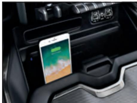
**CHARGING SOLUTIONS.** The front of the center console houses an auxiliary input and two sets of USB connections (Type-A/C pairs). There is also a phone shelf to hold smartphones with an optional integrated wireless charging pad.
