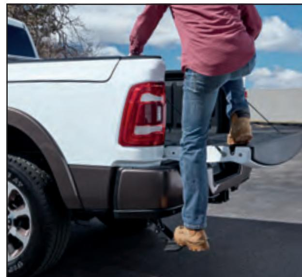
**BED STEP.** The available foot-actuated Mopar® Bed Step eases access to the bed and hides out of sight when not in use. Available as a factory-installed option or as a stand-alone Mopar Accessory.
