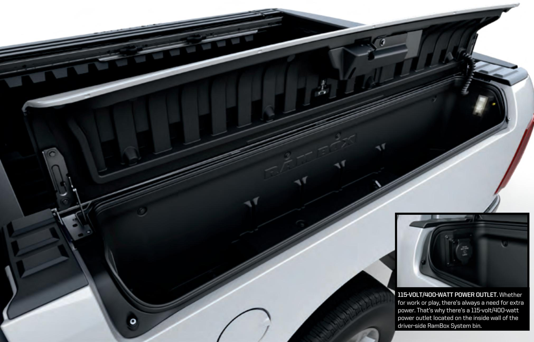
**115-VOLT/400-WATT POWER OUTLET.** Whether for work or play, there's always a need for extra power. That's why there's a 115-volt/400-watt power outlet located on the inside wall of the driver-side RamBox System bin.
