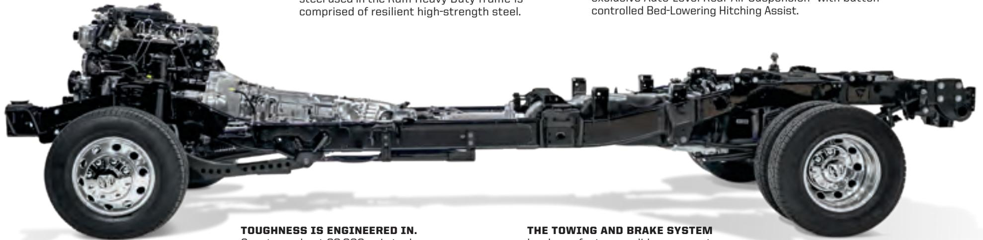
**TOUGHNESS IS ENGINEERED IN.** Count on robust 63,000-psi steel for the crucial engine crossmember.
