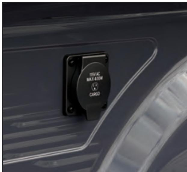
**BED OUTLET.** When you need power on the go, your Ram Truck is ready. Use the available 115-volt/400-watt power outlet located in the rear of the truck bed to plug in tools, lights or anything else you need to get the job done.
