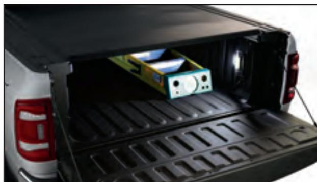
**IN-BED LED LIGHTING.** Controlled by a switch or activated when the unlock button on the key fob is pushed, the available side cargo-bed lights provide convenient illumination.
