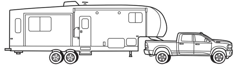
**FIFTH-WHEEL TOWING.** Capability comes from the fully integrated rear-axle crossmember on all frames. Available fifth-wheel hitch-mounting hardware is integrated into the production box floor—and includes fifth-wheel pucks.
