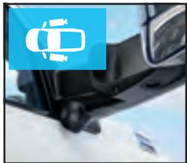
**TRAILER REVERSE GUIDANCE VIEW<sup>7</sup>** provides a single-screen view of both sides of the trailer and helps drivers more safely tow, park and maneuver long or short setups. The system stitches together select screens for simultaneous views of each trailer side; on-screen buttons give the driver left/right panning ability to better frame the trailer in the image. It's ideal for tight garages and parking spaces, and delivers fast, safe and efficient operation. No active lines are provided.
