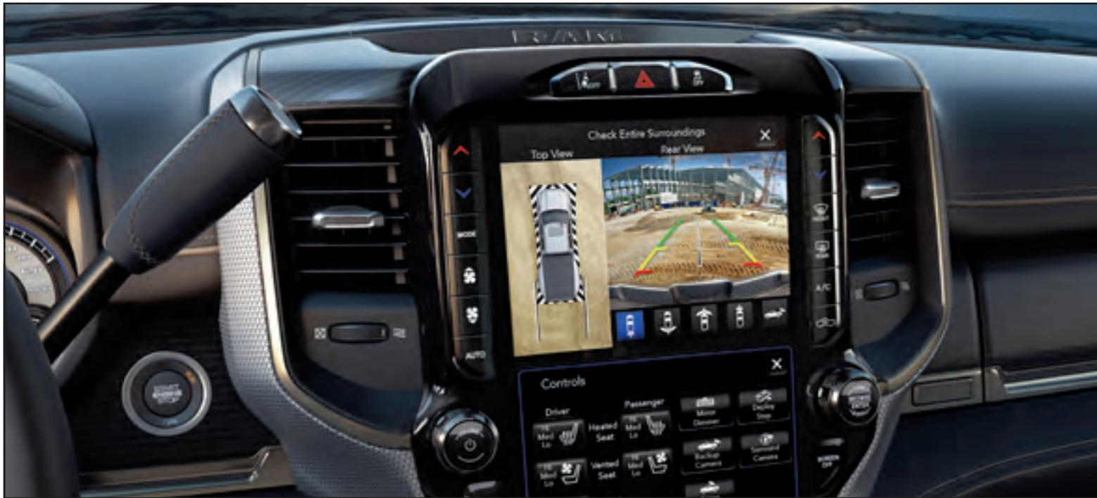
**THE AVAILABLE 360° SURROUND-VIEW CAMERA SYSTEM?** Thanks to strategically placed cameras—inside the front grille, in the outside mirrors and in the tailgate handle—you'll see a complete picture of the vehicle surroundings. The result is secure parking, loading/unloading and trailer hookup.
