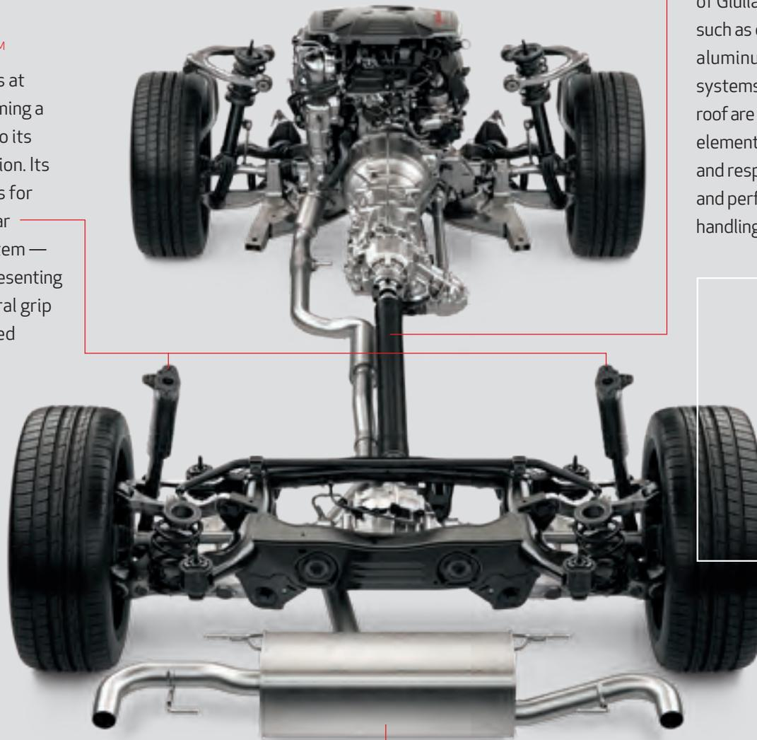
**CARBON FIBER DRIVESHAFT** An ideal power-to-weight ratio is the product of Giulia's lightweight, high-tech materials, such as carbon fiber for the driveshaft and aluminum for the engines, suspension systems, hood, doors and roof (hood and roof are carbon fiber on Quadrifoglio). These elements enhance Giulia's overall balance and response, providing excellent precision and performance — delivering exceptional handling even in extreme conditions.
