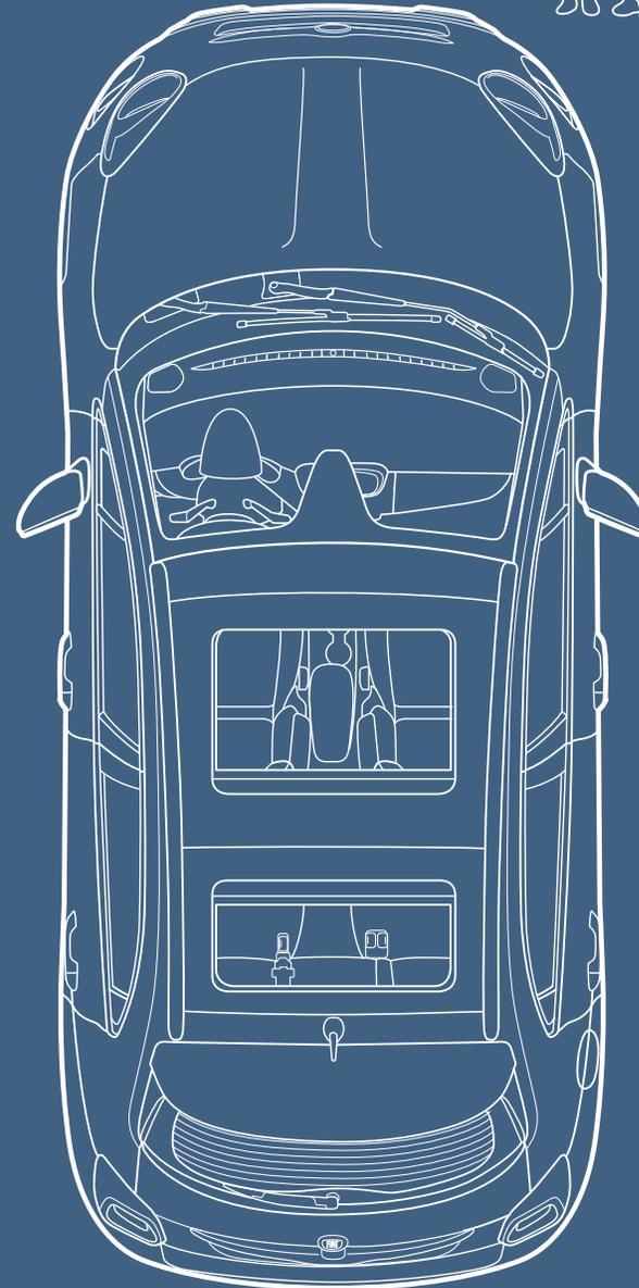
With a wheelbase of 101.2 inches, FIAT 500X measures 79.7 inches wide with mirrors extended, 63.7 inches tall and 168.2 inches long on Trekking models.
