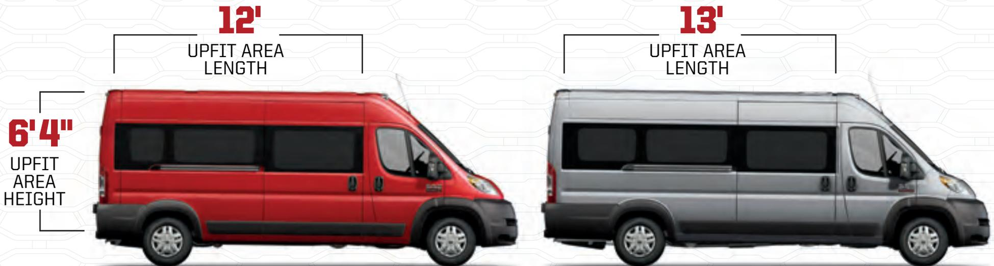
**ONE WHEELBASE, EXPANSIVE OPTIONS.** Utilize the extended body on Windowed Van to create a significantly larger interior. The 14.4-inch extension adds nearly 43 cubic feet of volume—the perfect solution when you need extra room for luggage or storage.
