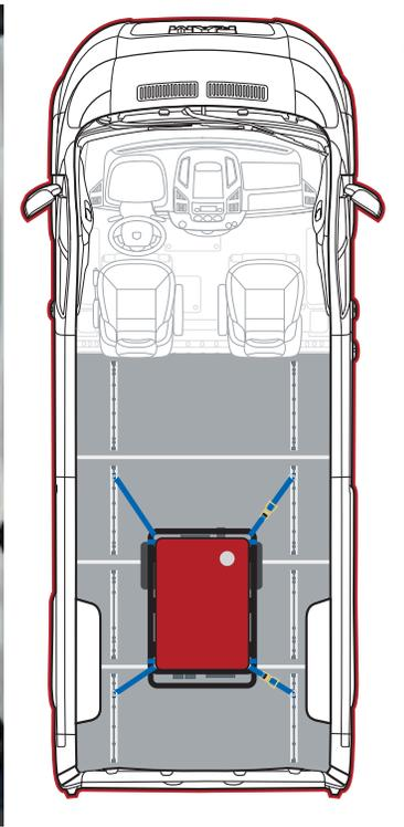
**CARGO TIE-DOWN TRACK SYSTEM.** This is multitasking at its best. The load floor system includes two in-floor tracks and two side tracks—one on each wall. Fitting all tracks are four 5/16-inch carriage bolts and four L-Channel Quick-Connect rings to securely strap down cargo—and they all work with the available shelving units as well. (Straps not included.)
