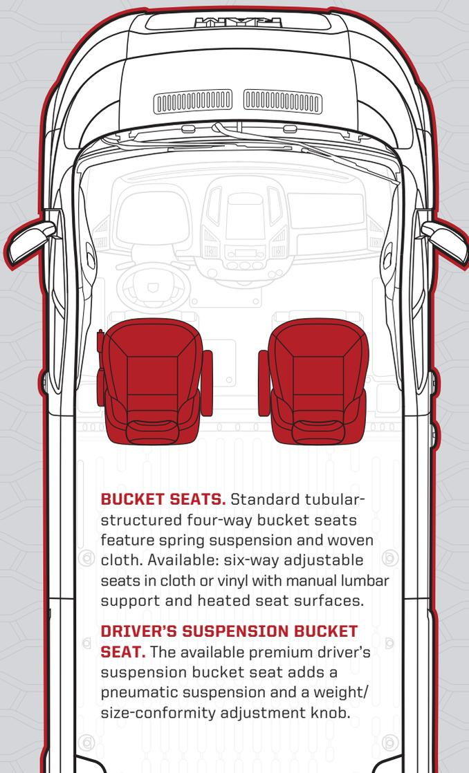
**BUCKET SEATS.** Standard tubular-structured four-way bucket seats feature spring suspension and woven cloth. Available: six-way adjustable seats in cloth or vinyl with manual lumbar support and heated seat surfaces.
