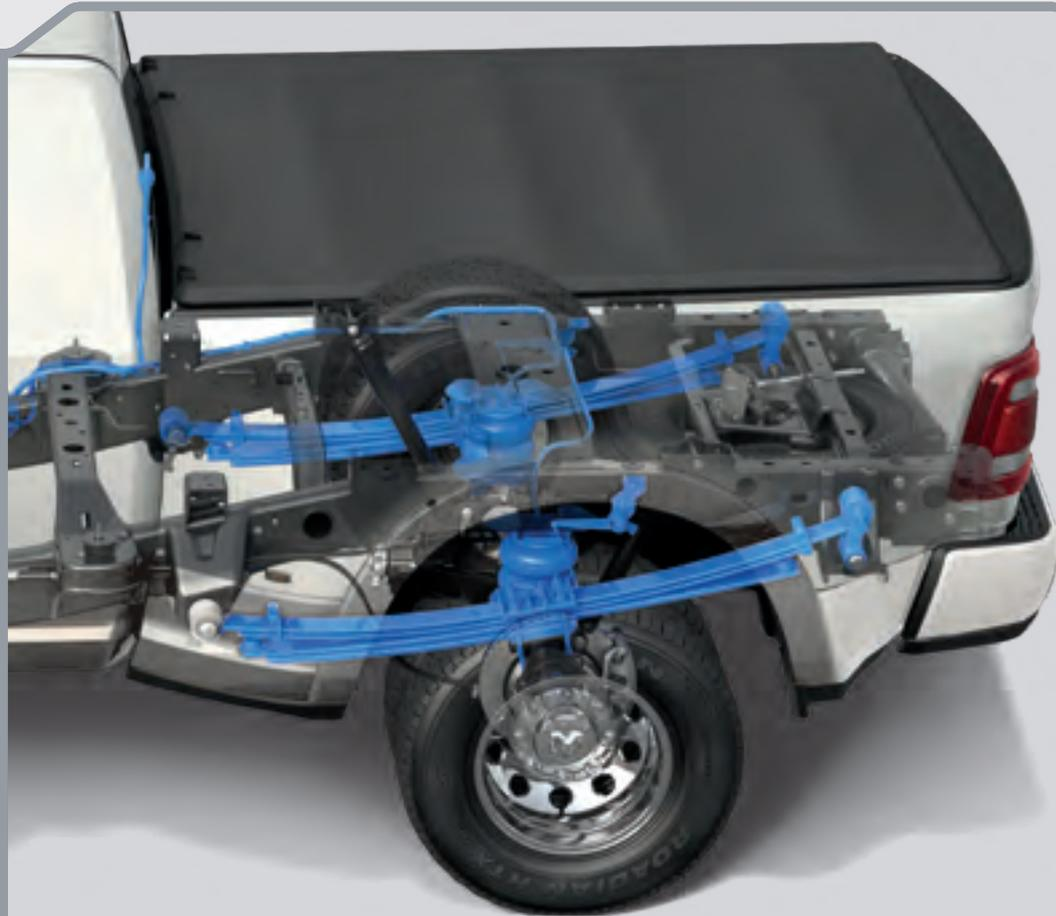
The Ram 3500 available Dual-Rear-Wheel Rear Air Suspension here shows how the leaf springs are augmented with the axle-mounted air springs.
