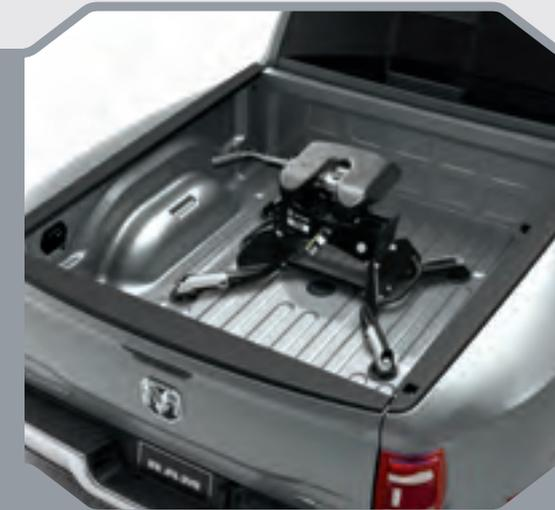
**GOOSENECK/FIFTH-WHEEL** varieties of towing rely on pure capability—starting with a strong rear structural crossmember. Note: along with the standard 4-/7-pin connector, the factory-installed Fifth-Wheel/Gooseneck Prep Group option includes an additional 7-pin connector integrated into the rear of the bed for easier access. When the Trailer Camera Prep Group is added, the 7-pin connector is upgraded to a 7-/12-pin connector.
