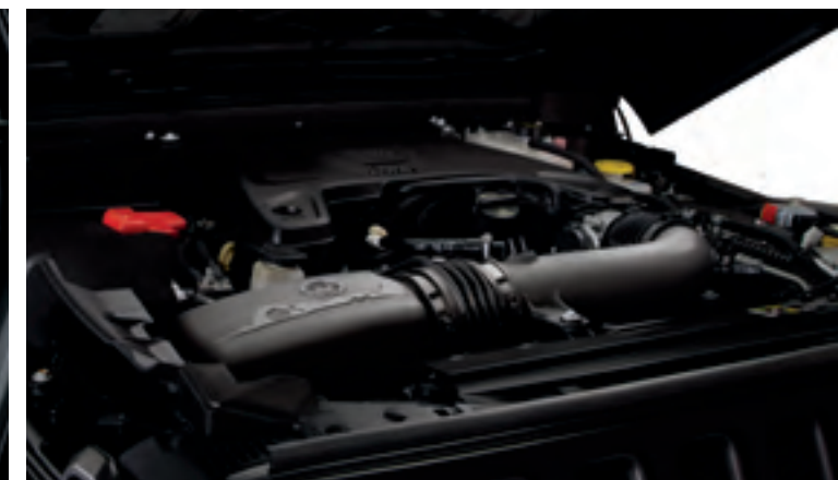
Cold Air Intake System 18
