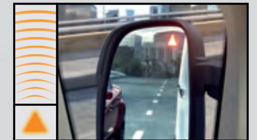
Available BLIND SPOT MONITORING (BSM) 3 with REAR CROSS-PATH DETECTION 2 AND SIDE-MIRROR NOTIFICATION SIGNAL LIGHT
